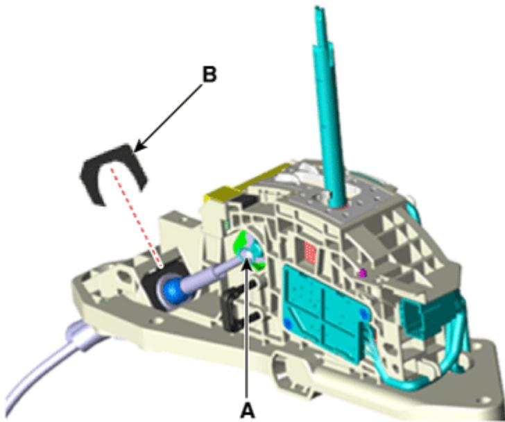
7. Remove the shift cable from the shift lever after loosening the screws (A).
