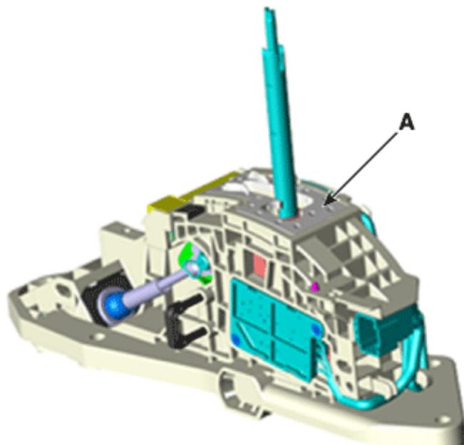
6. Remove the snap pin (A) and shift cable fixing clip (B).
